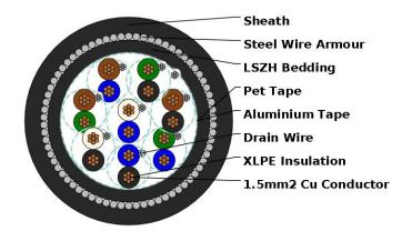
Application: The armoured LSOH versions (Part 1 Type 2) are generally used when the risk of mechanical damage is increased. The galvanised steel wire armour provides excellent protection. Generally used within industrial process manufacturing plants for communication, data and voice transmission signals and services, also used for the interconnection of electrical equipment and instruments, the LSOH sheath can reduce toxic smoke and fume emission.
