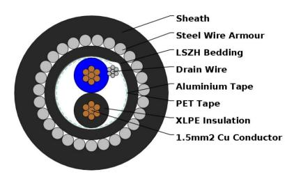
**Application:** The armoured LSOH versions are generally used when the risk of mechanical
