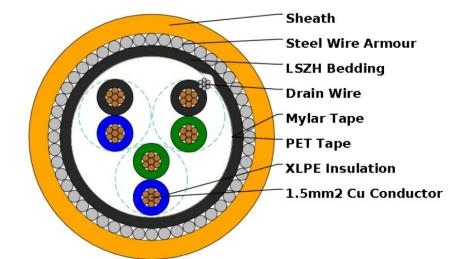
Application: The armoured LSOH versions are generally used when the risk of mechanical damage is increased. The galvanised steel wire armour provides excellent protection. Generally used within industrial process manufacturing plants for communication, data and voice transmission signals and services, also used for the interconnection of electrical equipment and instruments, the LSOH sheath can reduce toxic smoke and fume emission.
