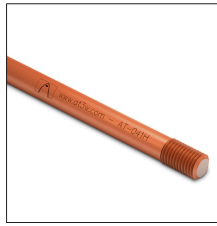
AT-041H ø5/8"x2m thrd 254µ Cu- bond earth rod
