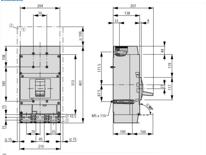
$oxed{1}$  Blow out area, minimum clearance to other parts: Ui  $\leq$  690 V: 100 mm
