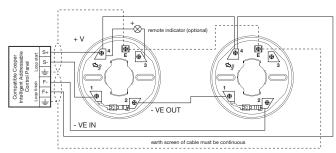
WARNING: If using the outer connection on terminal 2, ensure the operation of the switch is not impeded and that there are no shorts between terminal 2 and the switch contact.
