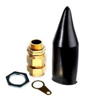
Brass indoor cable gland suitable for all types of steel wire armoured cable (SWA), providing mechanical cable retention and earth continuity via armour wire termination.
