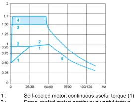
2: Force-cooled motor: continuous useful torque
