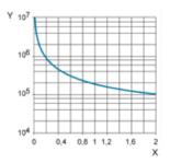
X Switching capacity (kVA) Y Durability (Number of operating cycles) Reduction coefficient for inductive AC load (depending on power factor cos φ)
