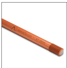
AT-041H ø5/8"x2m thrd 254µ Cu-bond earth rod
