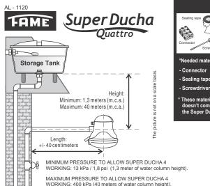
Minimum pressure to activate the appliance: 8kPa / 1 psi (0,8 meters of water column height).
