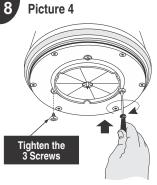
Once fitted in the Heating Chamber fix the Intermediary Base with 3 Screws using a screwdriver.
