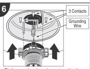
Fit the new heating element on the three contacts, being guided by the Guide Pin.
