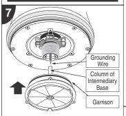
Before fixing the Intermediary Base, certify that the Grounding Wire is inside of the column of the Intermediary Base and your Garrison be fixed correctly.
