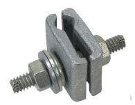
Lashing Wire Clamp is used for telco and CATV aerial plant to terminate and hold the end of the lashing wire, either at an interruption in continuity or at the end of the lashing wire coil. Also used to hang terminals and splice cases from strand.
