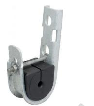
J hook cable clamp enable the direct suspension on cross arm poles of aerial optical cables with ADSS round structure and HDPE insulation,  $\emptyset$  5 to 17mm, deployed on distribution networks with spans up to 70m.
