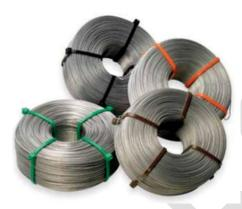
Stainless steel lashing wire is used in a lasher to lash a cable or combination of cables to a supporting strand. It is a specially controlled annealing process, which yields a uniform, fine grain strand structure thought the wire length.
