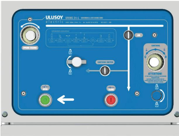
Push the opening (O) button to open load break switch.
