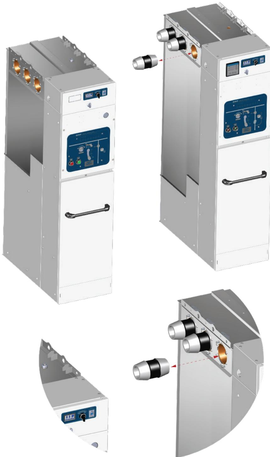
Modular Cubicles are combined by using 6 pieces of M8x30 bolt.
