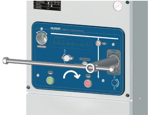
Rotate the lever in the direction of the arrow. **(Clockwise)**
