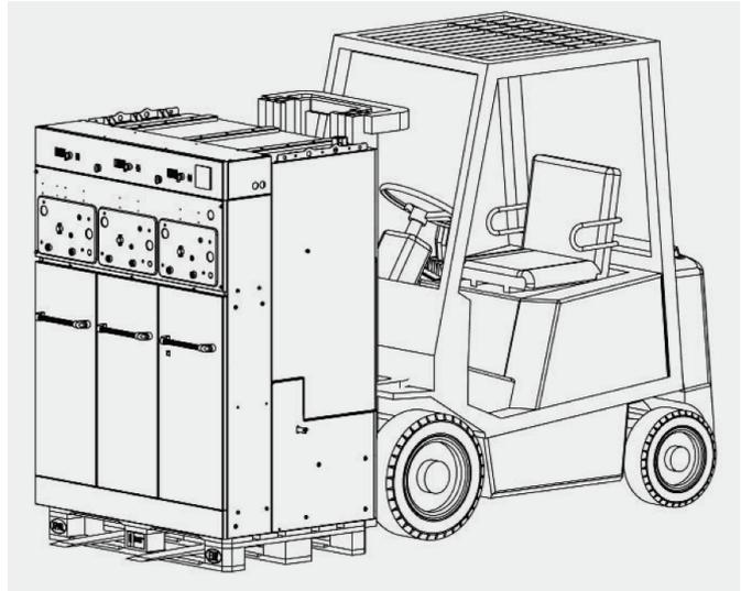
Lifting of a set of 3 **URING** functional units with a forklift truck
